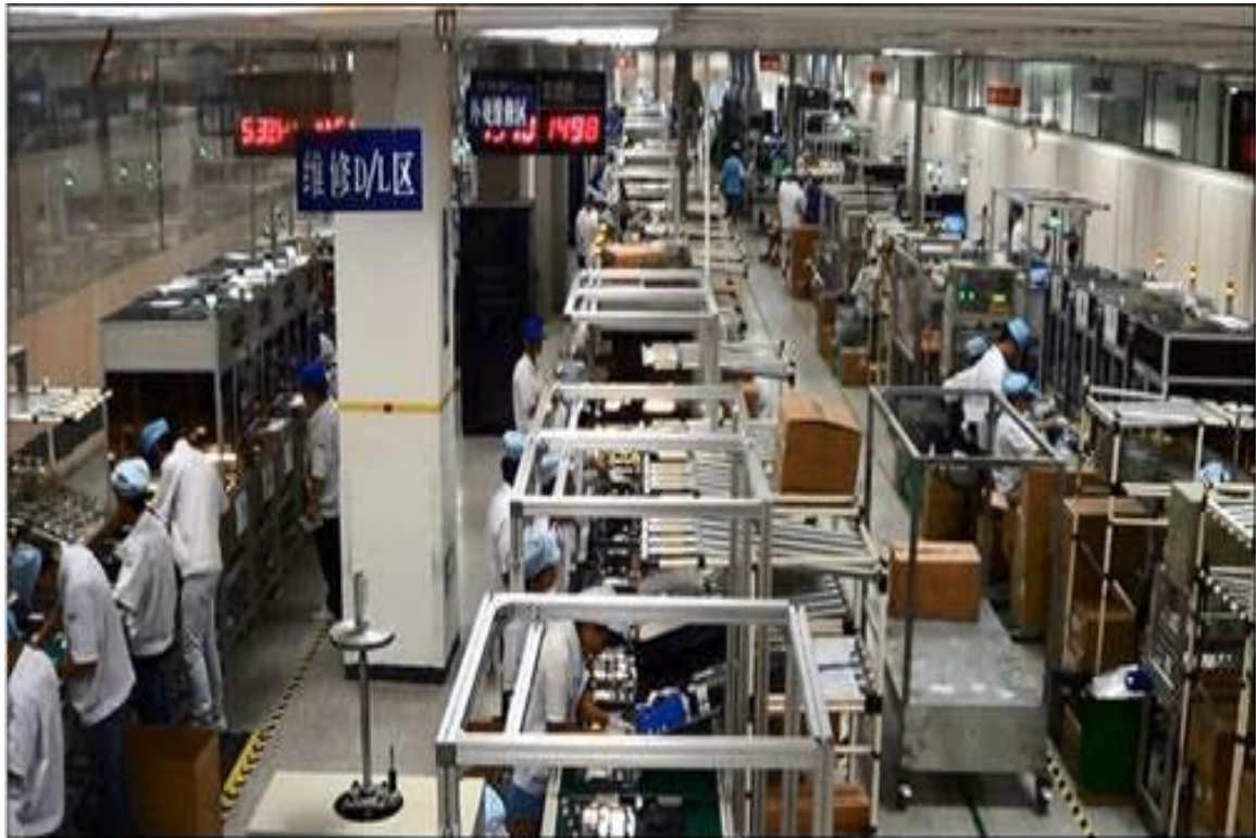
Figure 4. A new laptop assembly line comprised with robotic devices at many stations (those with metal frames) in Quanta, Chongqing in 2016 (Courtesy of Quanta). Thousands of assembly workers have been replaced by robotic arms and other automation devices.
