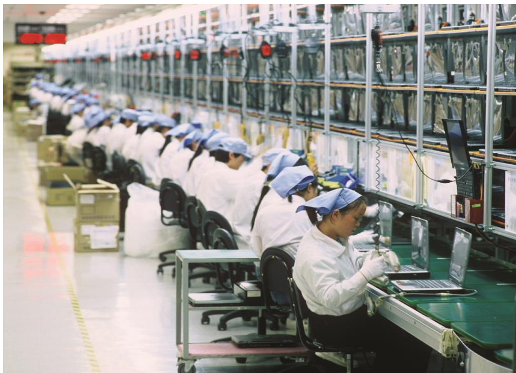
Figure 2. Operators and the flowing “run-in carousel” system in Quanta, Shanghai, 2007. It refers to the three moving levels of laptops up in front of the workers (Courtesy of Quanta).
